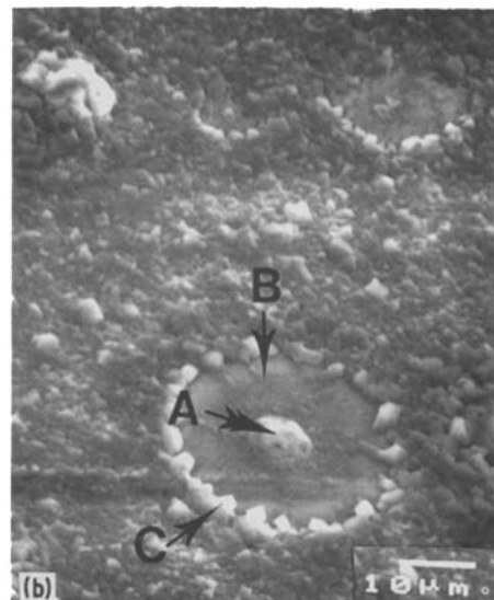
Figure 7 SEM of recrystallized sheet, electropolished surface, (a) after heating to 500°C in moist air and removing immediately; (b) same area after reheating to 500°C for 1 min showing Type 4 growths.
